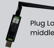
Plug Lora Module into lower middle USB port on Gateway
